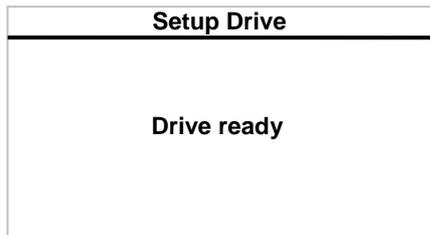
In the middle of the LCD is visualized the drive status.
